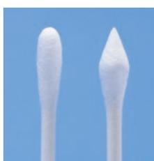
Single-use cotton swabs can be used in place of lens cleaning paper. The round type is suitable for cleaning large lenses and the cone type is suitable for cleaning small lenses or high-magnification objectives.
